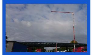
Ensure the GS6 pole is secured and weighted down if necessary. Check the pole is vertical, the cantilever pole is installed and the correct height assessment by the laser.
