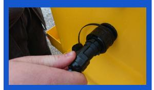
Connect GS6 connector to barrier, push down sleeve on barrier side and line up top single groove. Requires some force. Units with termination board
