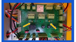
Check jumpers on internal control panel are in lower position. Safety OFF, GS6 ON.
