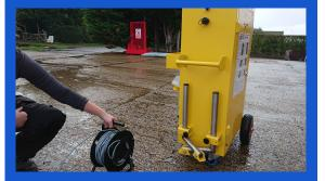
Extend cable reel to INSTABOOM barrier, ideally GS6 pole is at least 30m up lane of the barrier.
