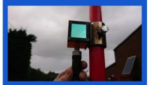
Line up connector to laser, screw connector to end of thread.
