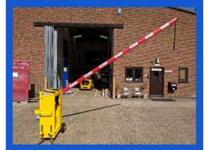
Test the operation of the unit. Raise barrier arm, block laser & test barrier lowers.
