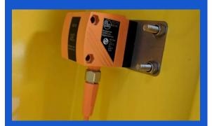
Disconnect the cable from the safety laser by unscrewing the metal collar and withdrawing the cable.
