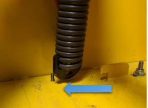
To move the mount position, move the barrier to the Up position, then slacken the bottlescrew until you can detach the spring from the hook at the bottom of the cabinet.
