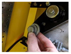
Once detached, unscrew the bolt and then bolt it into the appropriate hole on the spring arm. Ensure bolt is sufficiently tight.
