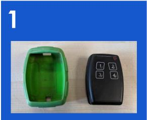
Unscrew the whip antenna and remove the device from the green boot
