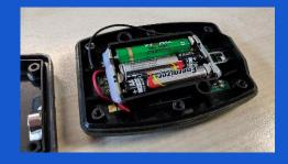
Exchange the three AAA batteries and reassemble the handset by reversing this process
