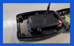
Open the case and remove the two black Philips screws from the battery case 4
