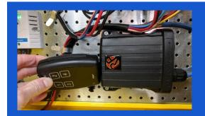
Touch the bottom left of the transmitter against the top left of the receiver for 1 second, as shown. The receiver will beep once. Press the chosen number switch on the transmitter you wish to pair. The receiver will beep twice to confirm pairing.
