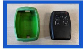
Unscrew the whip antenna and remove the device from the green boot
