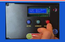
Open all units. First START SELF TEST..press SELECT. When all have successfully completed test they will read TEST COMPLETE.
